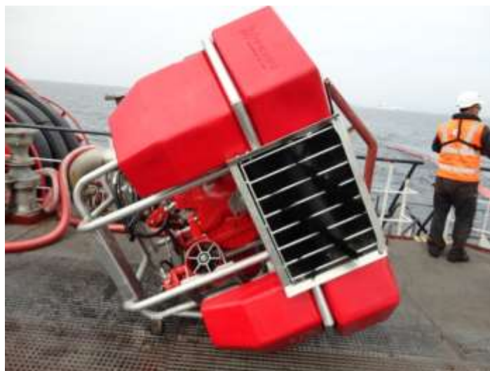
Fig. 20 NorMar 250 TI High Capacity Skimmer Set. Brush/disc skimmer head.
