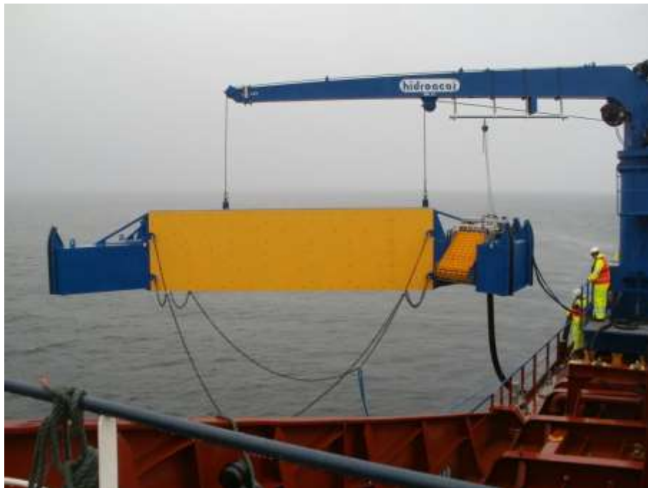
Fig. 1 LAMOR Stiff Sweeping Arm system LSS 12m
