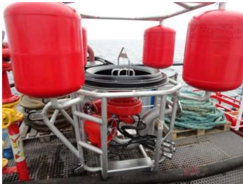
Fig. 22 NorMar 250 TI High Capacity Skimmer Set. Weir skimmer head.
