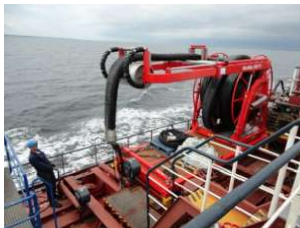
Fig. 25 Hydraulically driven reel with 360° turntable, umbilical hose and integrated crane
