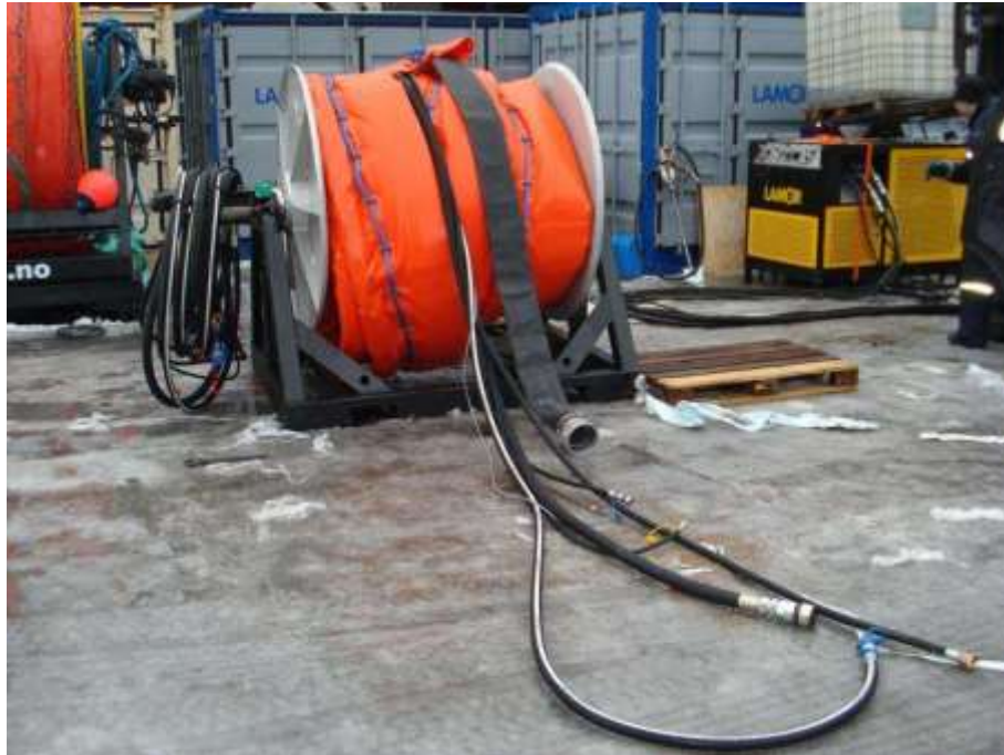
Fig. 11 Hydraulic and Oil Hose Set for LFF 400 W, on a hose winder
