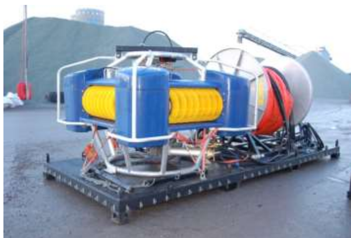
Fig. 13 Flat Rack Container 20' with the skimmer set
