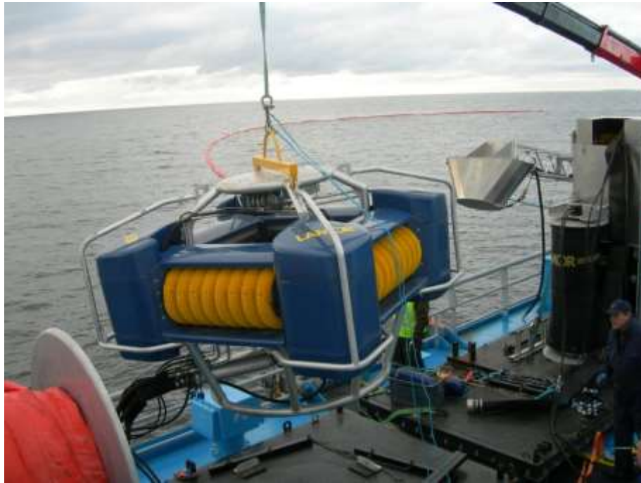
Fig.9 Brush Skimmer LFF 400 W
