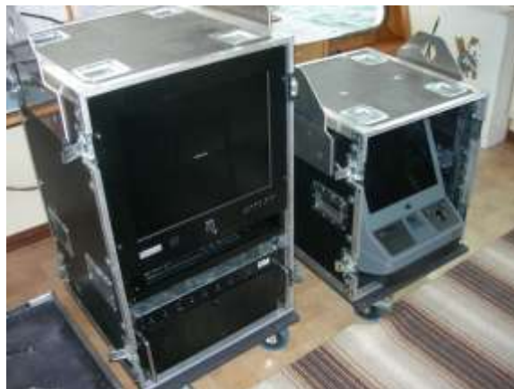
Fig. 31 SEADARQ Portable Oil Slick Detection System
