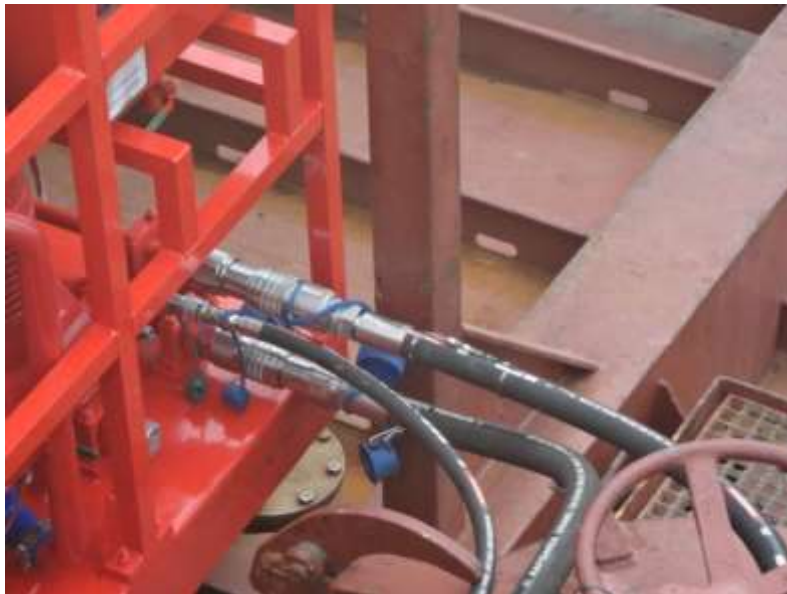
Fig. 28 Hydraulic hoses set connected to NorMar DHHP
