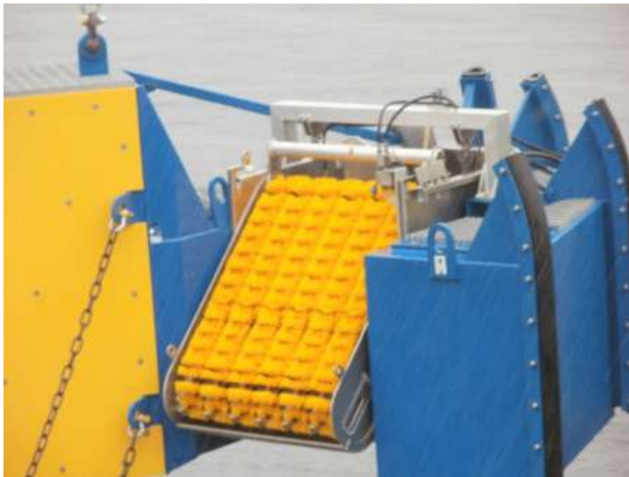
Fig. 2 LAMOR Stiff Sweeping Arm LSS 12m – brush skimmer module
