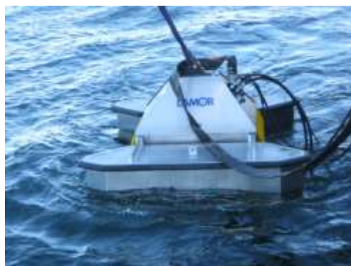
Fig. 14 Brush Arctic Skimmer LAS 125 W/P with floaters
