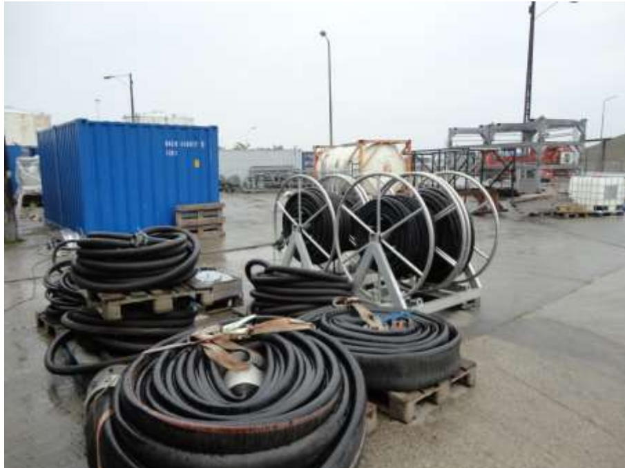
Fig. 7 2 Hose Winders LHW 40/2-AL with hydraulic hoses for LSS 12m
