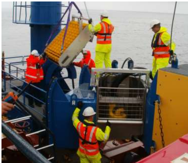
Fig. 3 LAMOR Stiff Sweeping Arm LSS 12m – weir skimmer module
