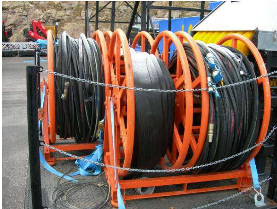
Fig. 17 Hose Winder for LAS 125 W/P Skimmer with oil and hydraulic hoses
